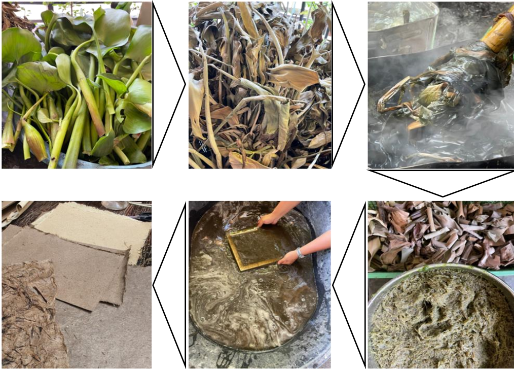
Figure 5. The process of making water hyacinth paper
