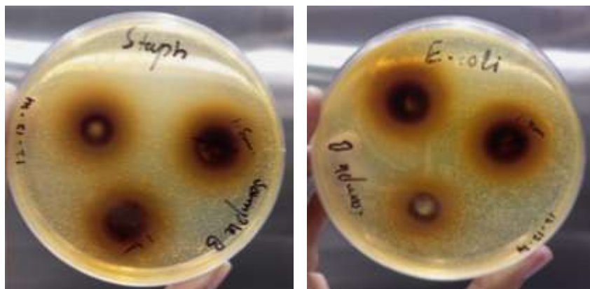
Figure 8. Asphaltum 2 against Staphylococcus aureus on the left and Escherichia coli on the right (Front side view)
