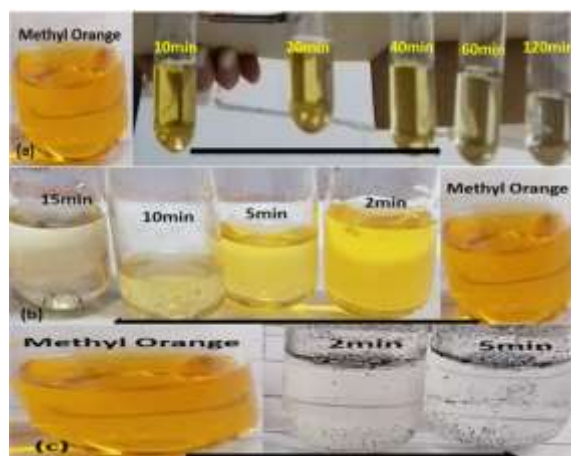
Fig. 9 Photocatalytic degradation of MO solution by using (a) 0.05 g, (b) 0.1 g, (c) 5 g of Ni doped CNTs (without acid)
