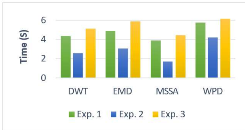
Figure 9: Comparison of computational time(s) between decomposition techniques using CNN based classifiers for noiseless data
