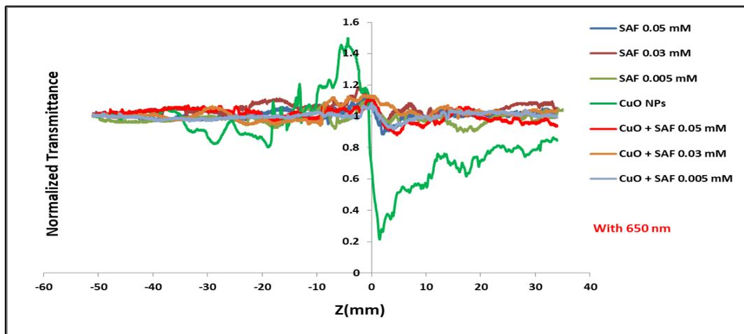
**Figure 17:** Nonlinear Refractive Index of Saffron Dye at Different Concentrations Before and After Addition of CuO Nps.
