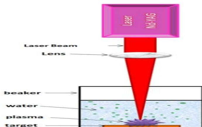
**Figure 1:** Experimental Setup for the Preparation of CuO Nps by Plal.
