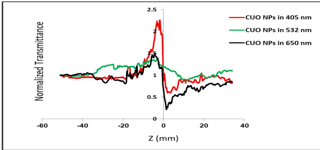
**Figure 6:** Nonlinear Refraction of CuO Nps With Effect of Three Wavelengths (405nm, 532nm, 650nm).
