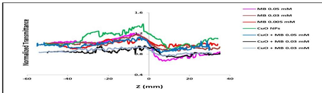
**Figure 13:** Nonlinear Refractive Index of Methylene Blue Dye at Different Concentrations Before and After Addition of CuO Nps.
