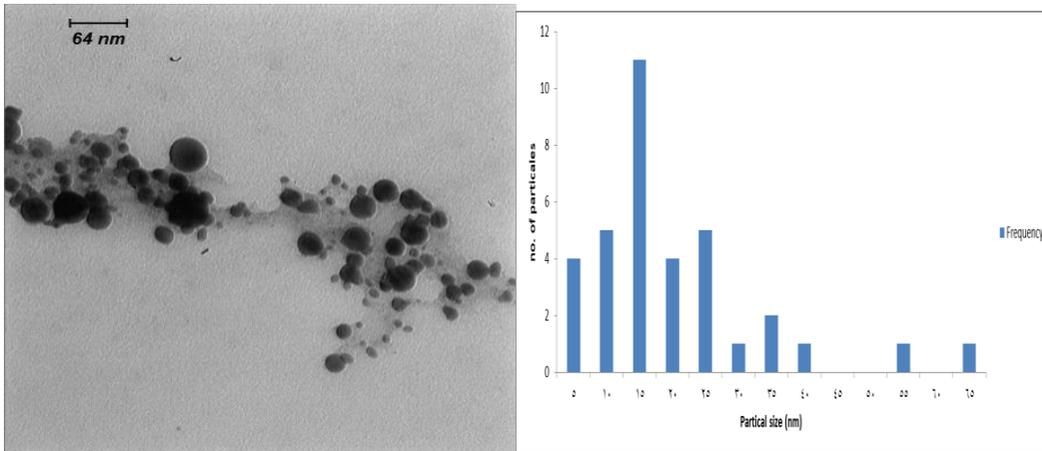
Fig 3: Tem Image of CuO Nps Synthesized by Laser Ablation in Distilled Water.
