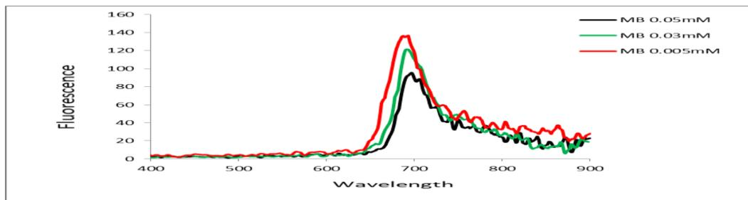
**Figure 10:** Fluorescence of Methylene Blue Dye at Different Concentrations.
