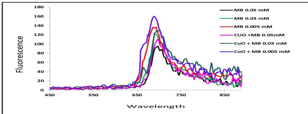
**Figure 11:** Fluorescence of Mb at Different Concentrations After Addition of CuO Nps.
