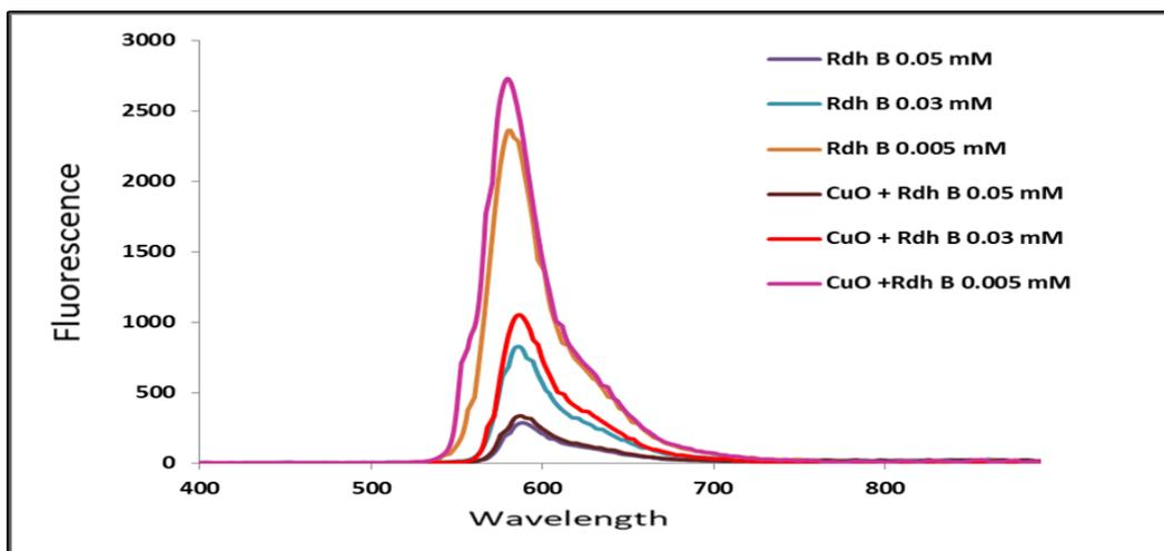
**Figure5:** Fluorescence of Rdh B at Different Concentrations after Addition of CuO NPs.
