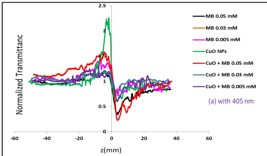
**Figure 12.:** Nonlinear Refractive Index of Mb Dye at Different Concentrations Before and After Addition of CuO Nps.
