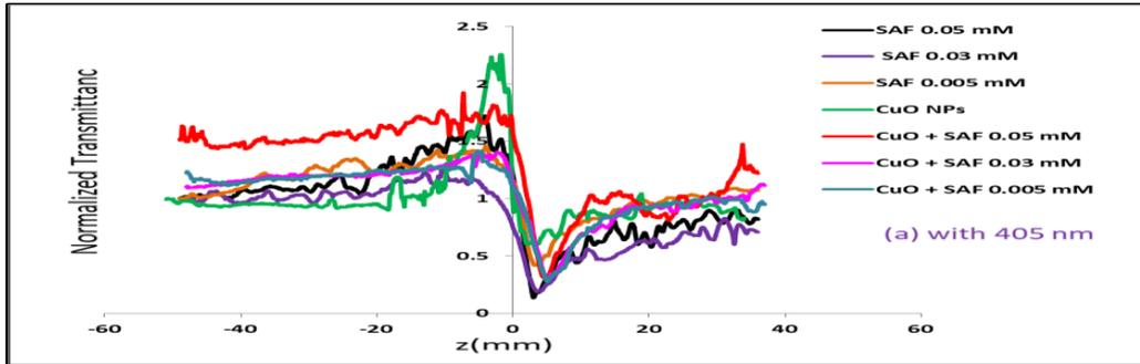
**Figure 15:** Nonlinear Refractive Index of Saffron Dye at Different Concentrations Before and After Addition of CuO Nps.
