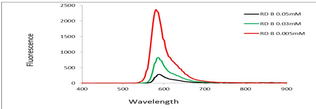
**Figure 4:** Fluorescence Spectra of Rhodamine B at Different Concentrations.
