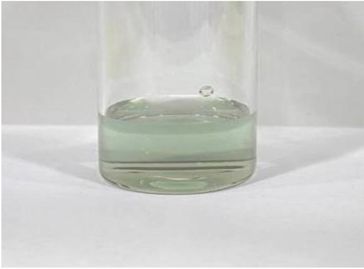
Figure 2: CuO Nanoparticles Produced by Laser Ablation in Distilled Water.
