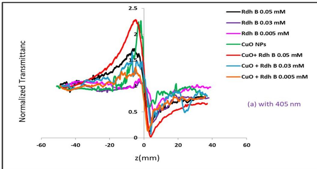
**Figure 7:** Nonlinear Refractive Index of Rhd B Dye at Different Concentrations Before and After Addition of CuO Nps.
