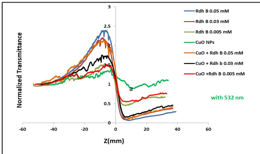
**Figure 8:** Nonlinear Refractive Index of R Rdh B Dye at Different Concentrations Before and After Addition of CuO Nps.
