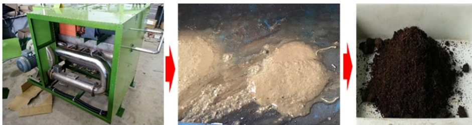
(Water Hyacinth and Wet Garbage Transforming Machine) (Transformed Wet Garbage from Household) (Finished Material Ready for Molding)
